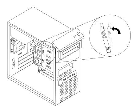
Figure 21. Removing the card reader retainer
